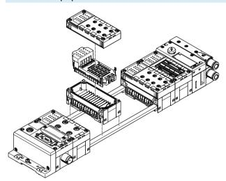
The mechanical connection between the CPX modules is established using tie rods. Two screws in the end plates are all that are needed to assemble the entire unit.
