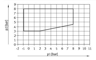
For valves in width 10 mm with code for position function 1-32: MU, NU, KU, HU
