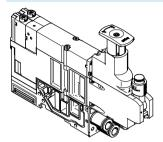
Additional functions can be added to each valve position between the sub-base and the valve.
