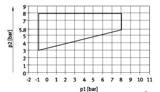
For valves in width 14 mm with code for position function 1-32: MS, NS, KS, HS, DS
